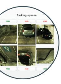
UPSOLUT sensors can monitor up to six parking spaces, three per each side of the aisle.
